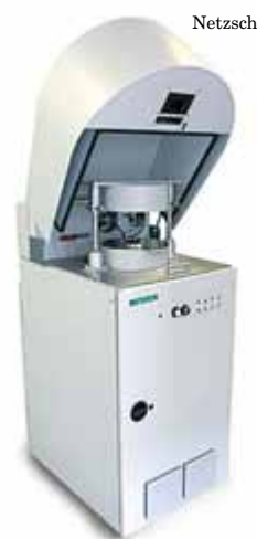
FIGURE 4. An accelerating-rate calorimeter (ARC) maintains isothermal conditions and can be used to determine the likelihood of runaway reactions
