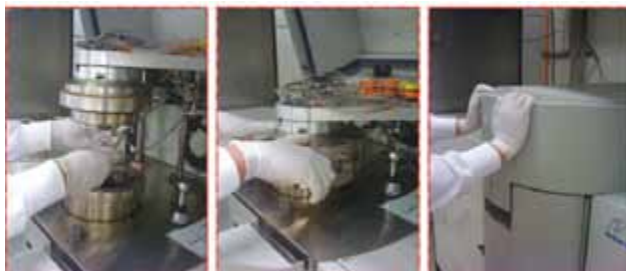
FIGURE 3. Adiabatic equipment, such as the APTAC, can be used to design safer work practices in reactive systems based on the determination of thermodynamic parameters over the whole reaction process
