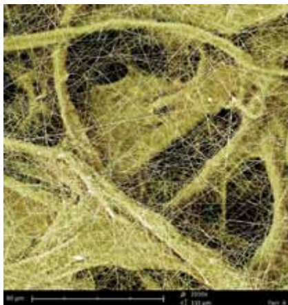
FIGURE 2. Shown here is the base media with a nano fiber coating as found in the HemiPleat eXtreme nano fiber filters, which offer high efficiencies
