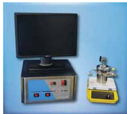
FIGURE 2. The Reactive System Screening Tool (RSST) can be used for a variety of tasks, such as designing emergency relief devices
