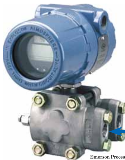
FIGURE 4. A biplanar connection has two ports on the side of the lower part of the unit. It supports gage, differential and absolute pressure measurements. It is heavier and more challenging to connect than in-line or coplanar designs
