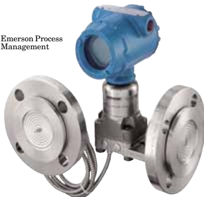
FIGURE 5. A remote seal and capillary system consists of external sensing diaphragms (which can be flush or extended, as shown) mounted to the process and connected to the DP transmitter either directly or via oil-filled capillaries
