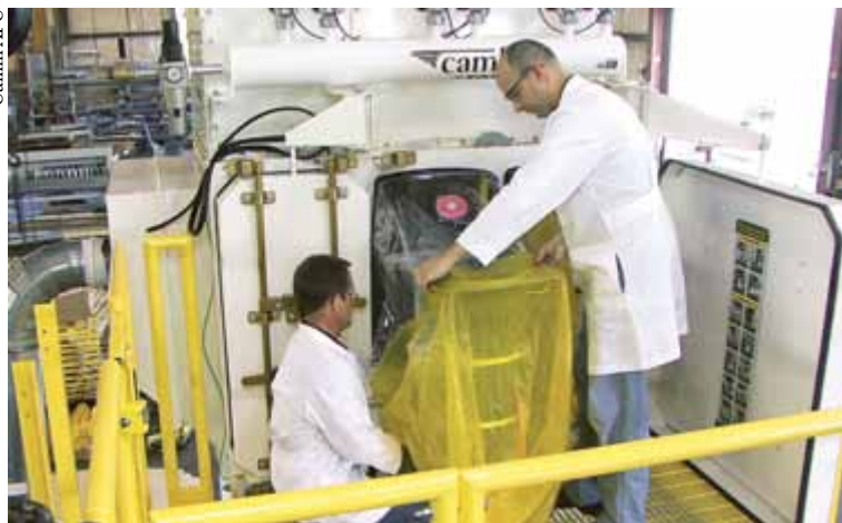
FIGURE 1. The Farr Gold Series Camtain dust collector offers bag-in/bag-out filter change out to help keep employees safe during handling of potent dusts
